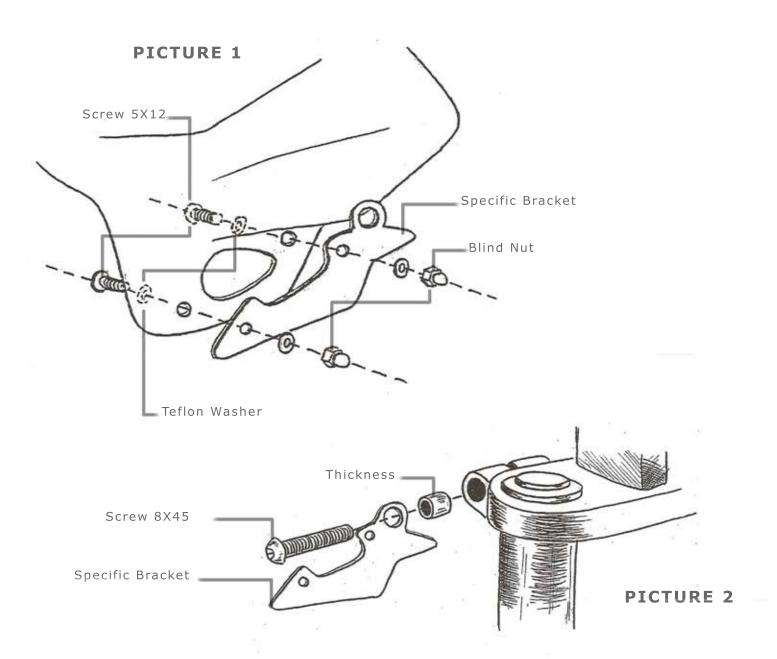
MOUNT THE BRACKET ON THE SIDE OF WINDSHIELD/SCREEN (PICTURE 1) REMOVE THE ORIGINAL HEAD-LIGHT UNSCREWING THE FOUR BOLTS ON THE SIDE. TAKE OUT THE INDICATORS FROM THEIR POSITION UNLOCKING THEM FROM THE INSIDE, TAKING OUT THEM FROM THEIR PLASTIC SUPPORT. DISCONNECT THE 2 CABLES.
